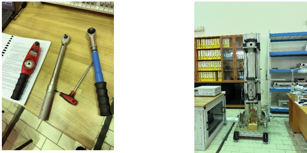
Figure 9 Hand Torque Tools and The Torque Calibration Machine
